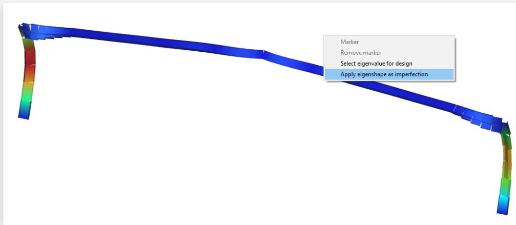
The new automatization, in case each load combinations, defines the proper direction of the imperfections and apply them accordingly during the analysis.
