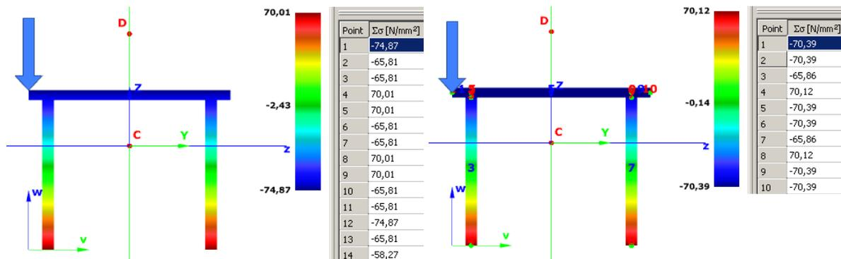
**Fig.13** Elastic stresses in the W7 welded hat section by the GSS and the EPS model
