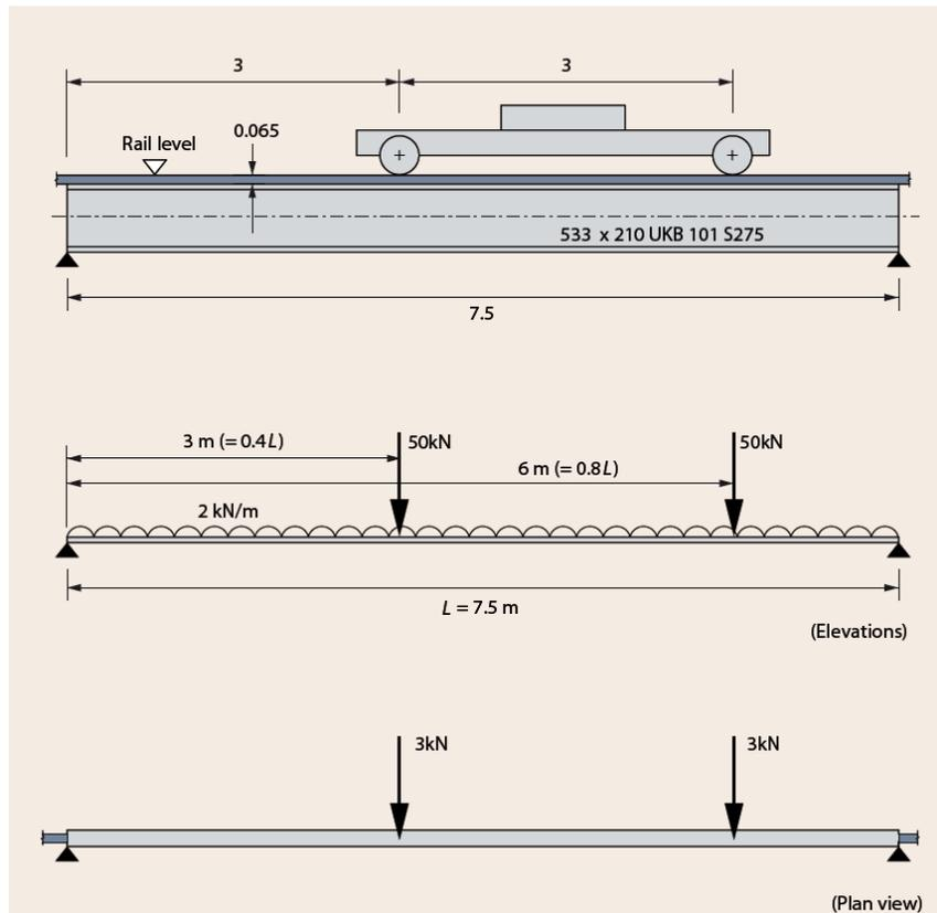
*Fig.68 Crane beam subject to two wheel loads*
