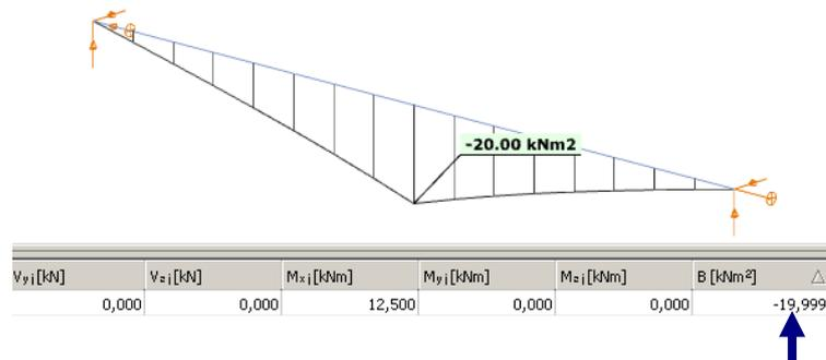
Fig.35 Bimoment of the member due to concentrated twist moment
