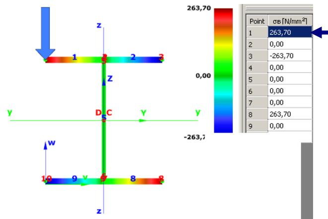
Fig.36 Warping normal stress in the middle cross-section
