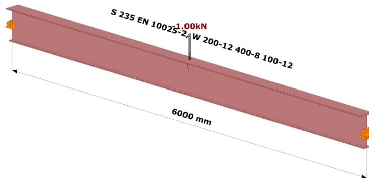
**Fig.55** Simple fork supported member with mono-symmetric welded I section subjected to transverse force (LTB)
