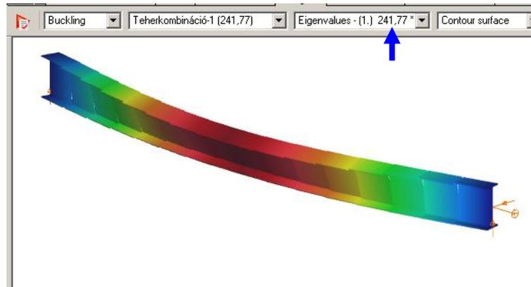
**Fig.49** LTB of simple supported structural member ( $n=16$ )
