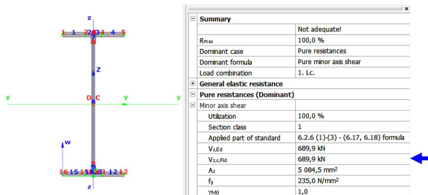
Fig.20 Design shear resistance of the IPE450 section
