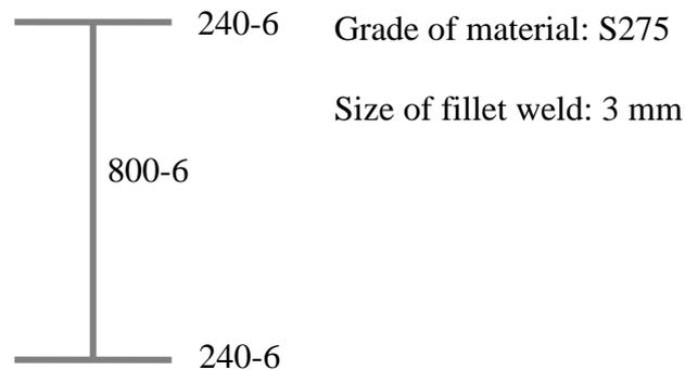
**Fig.9** Class 4 double symmetric welded I section (**W5**)
