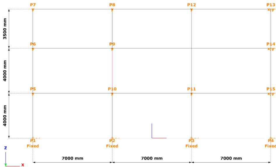
*Fig.78 Support of the non-sway frame*
