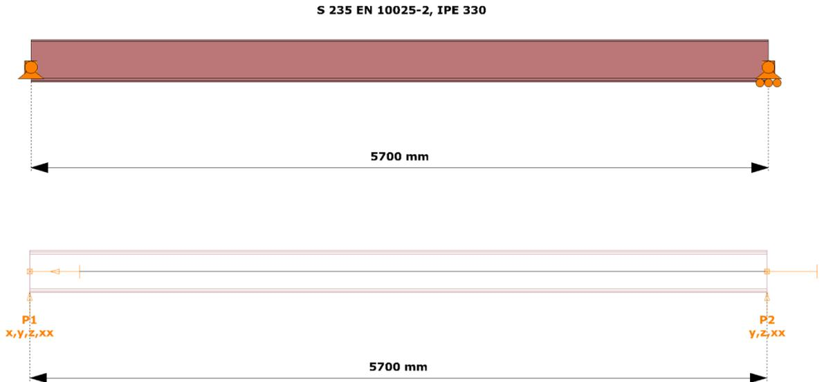
*Fig.70 Simply supported beam*
