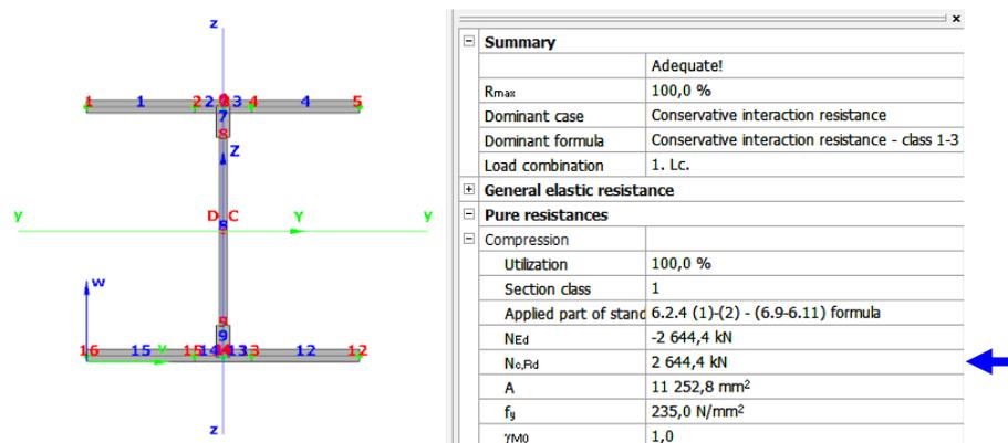
Fig.14 Design resistance of HEA300 section for compression
