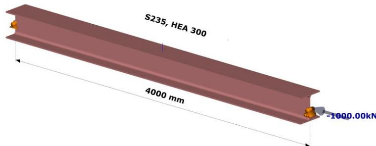
**Fig.26** Stress analysis of compressed member
