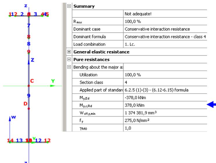
*Fig.18 Design resistance of the W5 welded Class 4 section for bending about major axis*
