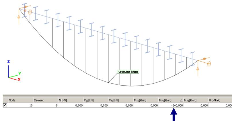
**Fig.31** Bending moment diagram of the bended member
