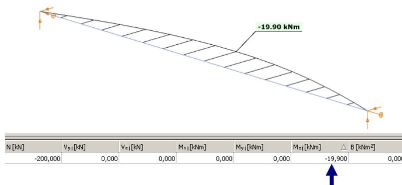
**Fig.44** Bending moment diagram of the member (n=16)
