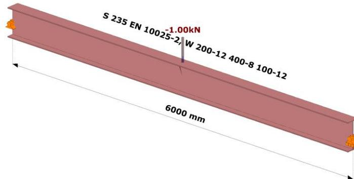
**Fig.50** Simple fork supported member subjected to transverse force (LTB)
