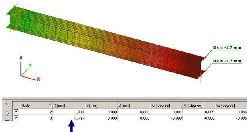
**Fig.28** Axial deflection of the compressed member
