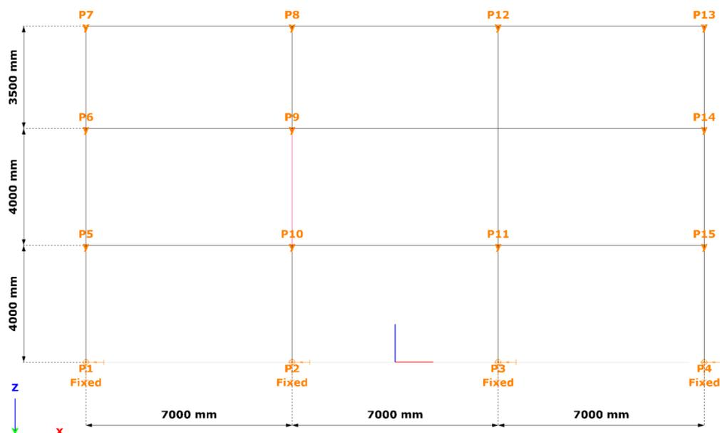
*Fig.36 Support of the sway frame*
