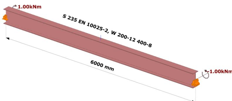
**Fig.48** Simple fork supported member subjected to bending about the major axis (LTB)
