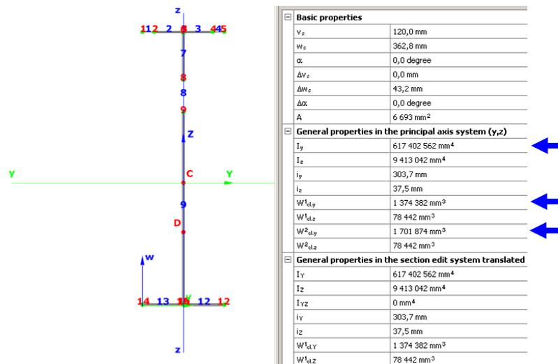
**Fig.10** Effective EPS model of the W5 section due to bending about major axis
