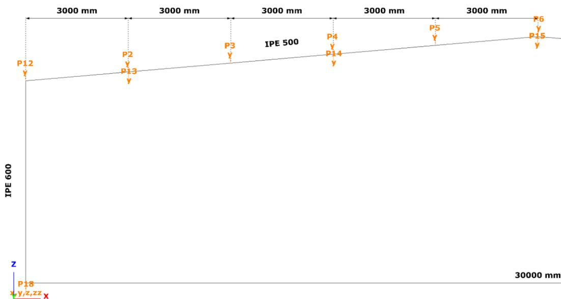
*Fig.75 Torsional restraints*
