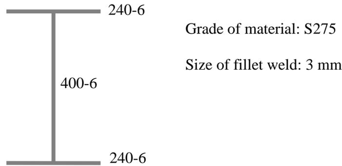
*Fig.7 Class 4 double symmetric welded I section (W4).*
