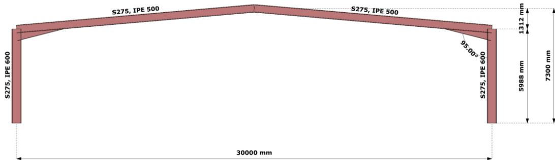
*Fig.74 Single bay portal frame with hot-rolled sections*
