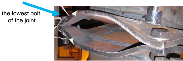
Figure 6. Joint after test TE1
