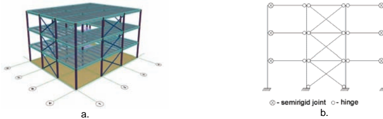
Figure 6. Reference structure (a) and structural model frames with bracings (b)
