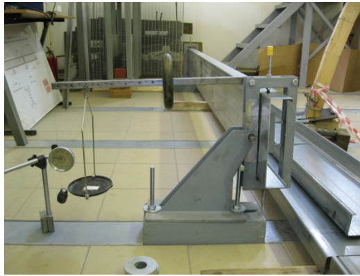
Figure1. Uniform torsion experimental set.
