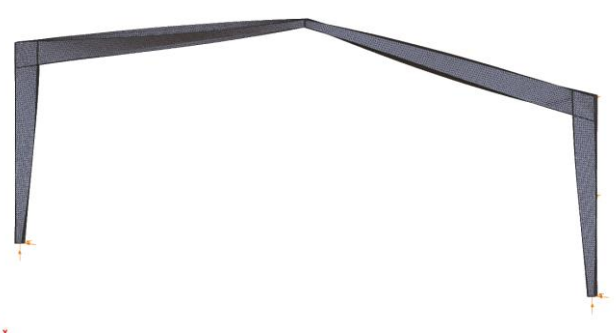
Fig. 11. Buckling mode by FEM (shell3)
