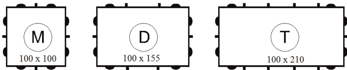
Fig. 2. The considered upright cross-sections (dimension in millimetres).
