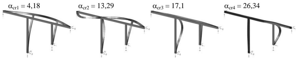
Figure 3: Case2 – first four eigenmode and eigenvalue.
