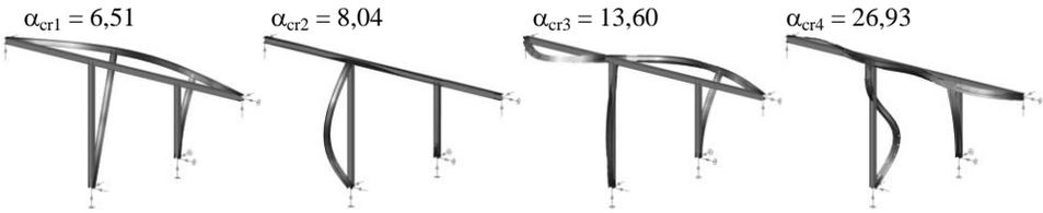
Figure 4: Case3 – first four eigenmode and eigenvalue.
