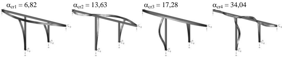
Figure 5: Case4 – first four eigenmode and eigenvalue.
