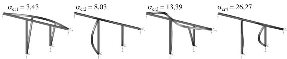
Figure 2: Case1 – first four eigenmode and eigenvalue.
